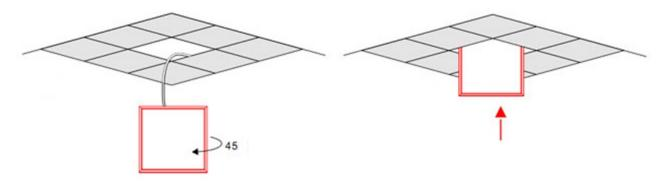
4. Attach cables to panel and place in ceiling grid. Adjust cables to remove slack until fixture is flush with drop ceiling tiles.
