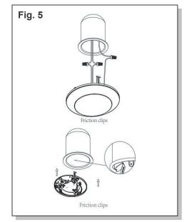
Push the LED fixture into the recessed housing until the trim ring is flush with the ceiling. (Fig. 5) **Note:** When mounting to a textured, popcorn, or uneven surface, use a silicone sealant to ensure a waterproof seal.
