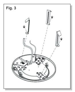
Attach the three friction clips to the mounting plate with screws provided. (Fig. 3)
