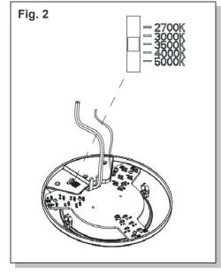
1. Before installation, select your preferred CCT by moving the switch to either 2700K, 3000K, 3500K, 4000K or 5000K. (Fig. 2)
