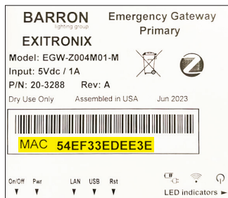
Figure 1: Example MAC address sticker located on the face of a gateway device. The MAC address is highlighted in yellow. In this instance, for a standalone gateway configuration, the Wi-Fi network the user should connect to is: "LYNXUS_ZGW-EDEE3E". Additionally, the associated gateway password in this case would be: "EDEE3E"
