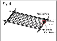
5. Open the fixture J-box by removing the access plate and make electrical connections inside (Fig. 5 and Electrical Connections section). Make sure to firmly secure conduit to the access plate before replacing the access plate to the fixture J-box when complete.
