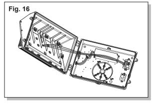
6. Reattach the fixture cover by sliding the cover over the pins in the fixture base. Reconnect the wire harness. (Fig. 16)
