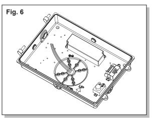
6. Feed the load wires through the center hole in the fixture base. (Fig. 6)
