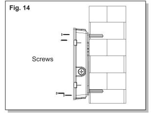
4. Secure the fixture base to wall using appropriate hardware for the mounting application (provided by others). (Fig. 14)
