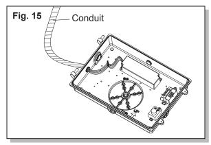
Attach conduit to the fixture base. Refer to the wiring diagram for electrical connections. Use wire nuts (provided by others) for connections. (Fig. 15)
