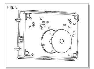
5. Attach the gasket pad to the backside of the fixture base. (Fig. 5)
