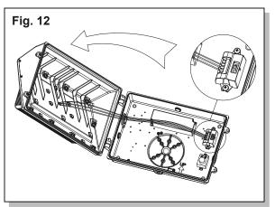
2. Swing open the fixture, disconnect the wire harness, and remove the front cover. (Fig. 12)
