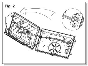
2. Swing open the fixture, disconnect the wire harness, and remove the front cover. (Fig. 2)
