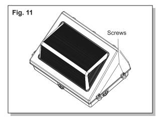
1. Remove the screws from the side of the fixture and set aside. (Fig. 11)
