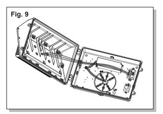
9. Reattach the fixture cover by sliding the cover over the pins in the fixture base. Reconnect the wire harness. (Fig. 9)
