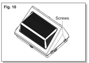
10. Tighten the screws to secure the fixture cover to the base. (Fig. 10)
