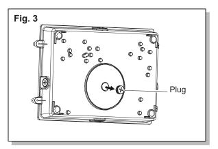
3. Unscrew and remove the plug from the fixture base. (Fig. 3)
