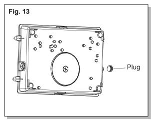
3. Unscrew and remove any one of the four (4) side plugs. Attach the gasket pad to the backside of the fixture base. (Fig. 13)
