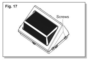
7. Tighten the screws to secure the fixture cover to the base. (Fig. 17)
