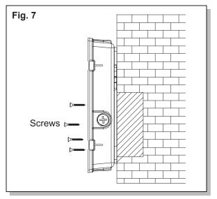
7. Secure the fixture base to J-box using screws (provided by others). (Fig. 7)
