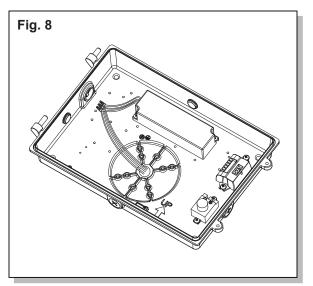
8. Refer to the wiring diagram for wiring connections. Use wire nuts (provided by others) for connections. (Fig. 8)
