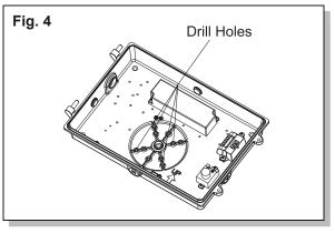
4. Drill holes in the fixture base with the same hole pattern as the J-box. (Fig. 4)
