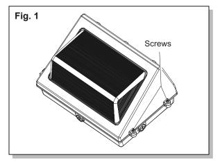
1. Remove the screws from the side of the fixture and set aside. (Fig. 1)
