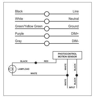
Note: This fixture auto adjusts for voltages from 120-277V or 347-480V driver. Cap all unused leads to prevent shorting.
