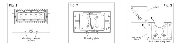
**IMPORTANT:** Weatherproof your outdoor installation, be sure to seal all holes in the fixture's housing such as the mounting, conduit, plugs, sensors, photocontrols, etc. with silicone sealant.
