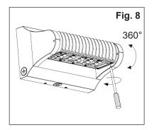
**IMPORTANT:** Weatherproof your outdoor installation, be sure to seal all holes in the fixture's housing such as the mounting, conduit, plugs, sensors, photocontrols, etc. with silicone sealant.
