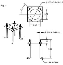
2. Install anchor bolts in concrete. Pass electrical wires through center hole in anchor bolt template.
