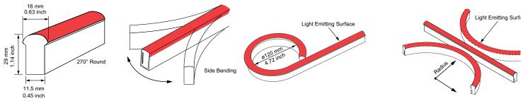
Minimum Bending Diameter 4.72" (120mm)
