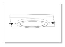
Align the light slots with the mounting bracket slots and secure with plastic push-in clips. Press light flush with surface and install optional magnetic trim ring if compatible.
