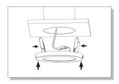
5. Press friction clips inward and insert clips into can housing.
