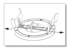
3. Install light to mounting bracket and secure with plastic push-in clips.
