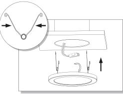
Squeeze torsion clips and insert into existing can housing torsion clip mounts.
