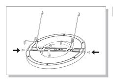
4. Install light to mounting bracket and secure with plastic push-in clips.
