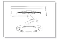
Make wire connections (see Wiring diagram). Set color switch if equipped.
