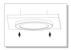
Press light flush with surface and install optional magnetic trim ring if compatible.
