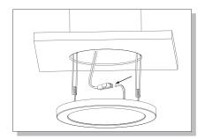
insert wires into adapter connector per wiring diagram. Set color switch if equipped.
