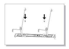
3. Install torsion clips to mounting bracket with provided screws.
