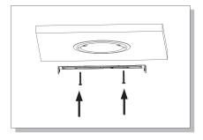
1. Install the mounting bracket to the J-box with provided hardware.
