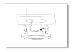
Insert light wires into adapter connector, make wiring connections per wiring diagram. Set color switch if equipped.
