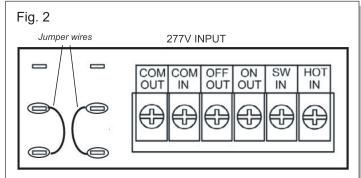
**NOTE:** Factory terminated jumper wires are provided with Mesa systems for making user selected input/output voltage connections.
