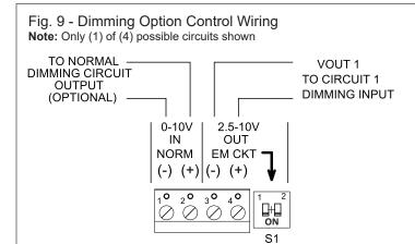
**CAUTION:** The sum of the dimmed load levels for all circuits combined must not exceed unit rating in emergency mode.
