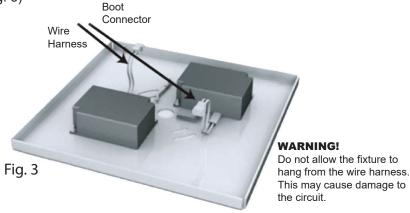
5. Mount bottom enclosure to the cover plate with (4) screws.
