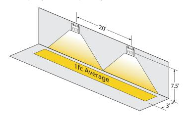
Using multiple units mounted at a typical 7.5' height delivers 20' on center spacing with a 6' wide path of egress.
