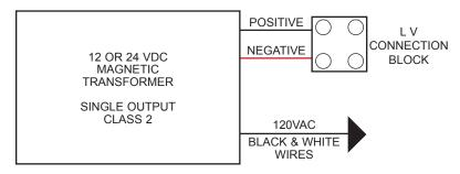
This is a transformer-based power supply. To dim, use a Low Voltage Magnetic Dimmer on the Primary.
