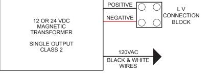
This is a transformer-based power supply. To dim, use a Low Voltage Magnetic Dimmer on the Primary.
